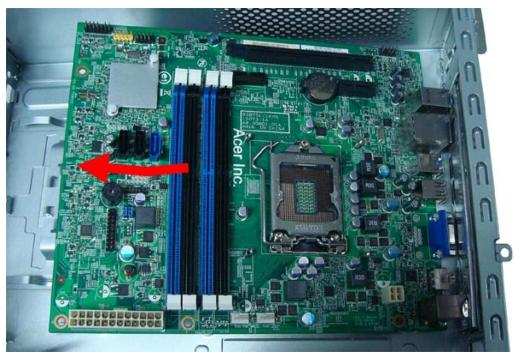
3. Punching in IO Shield then you can remove it.
